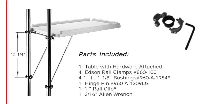
Assemble the clamps #860-100 around the pedestal guard tubes. Two clamps on each tube 12 1/4" apart with the horizontal holes forward.
