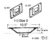
Side Inlet Nitrile Pump Spares Kit Order # 114N-117-120 Includes: 113N-0 Size 0 Diaphragm - Nitrile 160-G-107 Valve Assembly - Nitrile(2) 160-A-1200 3/8" Sealing Washer - Stainless (2)
