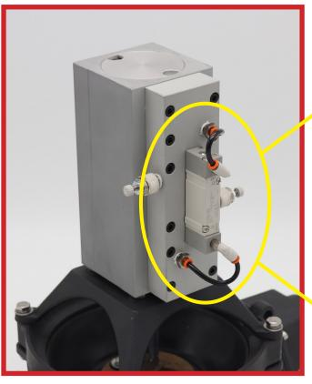
You can see the first release valve looking down from the top of the pump and the second by looking upward from the bottom of the pump. With one pen or paper clip (something small enough to press in the button), press one of the release valves, clearing the Air Motor and allowing the pump to be operational again!
