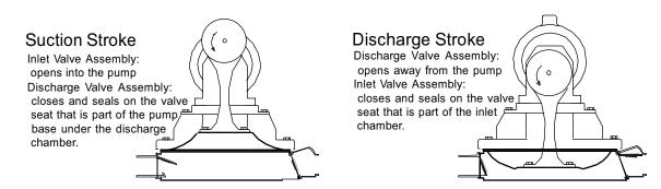
**Diaphragm:** Edson 120 Pumps use Elastomer Diaphragm and Flapper Valves. Over time these parts wear and need to be replacement. The ability to easily and quickly replace these inexpensive parts is one of the major advantages of an Edson diaphragm pumps. Edson has packaged these parts as Spares Kits. See the parts list for the order #s.
