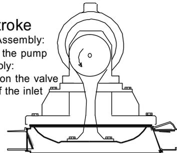
**Diaphragm:** Edson 120 Pumps use Elastomer Diaphragm and Flapper Valves. Over time these parts wear and need to be replacement. The ability to easily and quickly replace these inexpensive parts is one of the major advantages of an Edson diaphragm pumps. Edson has packaged these parts as Spares Kits. See the parts list for the order #s.
