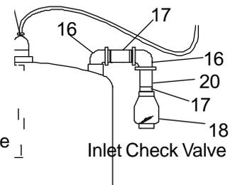
If a check valve is clogged, it may be removed for cleaning. The check valves are screwed in using regular NPT threads. Since the check valves are plastic, care should be taken while unscrewing them with a standard pipe wrench. It is a good idea to install two shutoff ball valves in front and behind the discharge check valve during installation. This insures a minimal amount of mess while removing the discharge check valve in the event that either the tank or the discharge line is full of waste.
