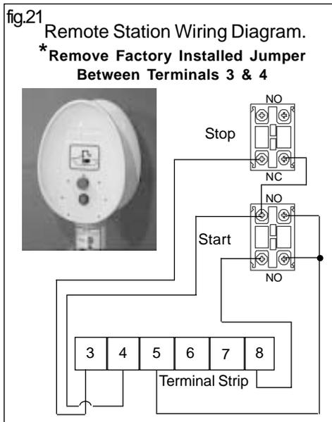
*Note: 4 wires are being used to wire the remote stations to the main panel terminal strip.*
