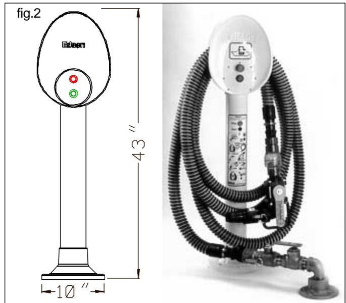
**Hydrant:** (Optional) 1 1/2" Bronze Check Valve, Ball Valve and Quick Clamp Hose Adapter with Bronze Elbow and Close Nipple with Mounting Flange. fig. 4
