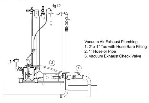
Positive Head Installations - When the vacuum tank outlet is below the place into where the tank is being emptied, the exhaust air line must be extended parallel to the discharge line and the connection made where the discharge line begins to gravity drain.
