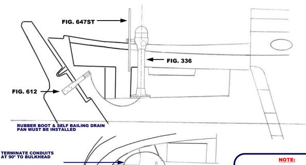
The best way to lead the conduits from the quadrant, and to be able to align them properly, is to cut out the tops of the seat outboard of the bulkheads which make the lazarette watertight. These openings would allow for the alignment & securing of the conduit ends. The seat tops would be removable so that inspection & service could be done.
