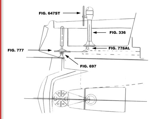
THE SCUPPER DRAIN ON SOME MODELS MAY HAVE TO BE MODIFIED IN ORDER TO HAVE THE RADIAL DRIVE WHEEL FIT.
