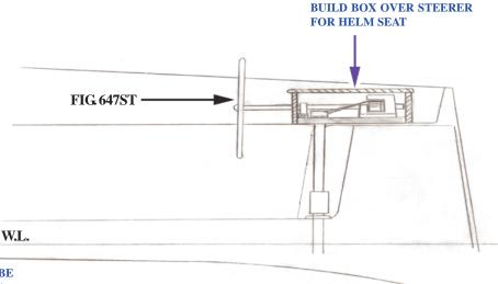
LARGE LAZARETTE HATCH TO BE SEALED & PROVISIONS FOR (2) SMALLER HATCHES TO ALLOW ACCESS TO LAZARETTE ON BOTH SIDES OF STEERER TO BE MADE
